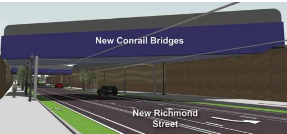
GR1 improvements include construction of four smaller bridges to replace the low-hanging Conrail overpasses on Richmond Street near Lehigh Avenue.
